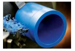
Plant and Maintenance Managers find that machining bearings to size from pre-grooved or standard Thordon tubes reduces their industrial bearing inventory and repair turn around times. The Thordon Bearing Sizing Calculation Program offers easy computer-based dimension calculations.
