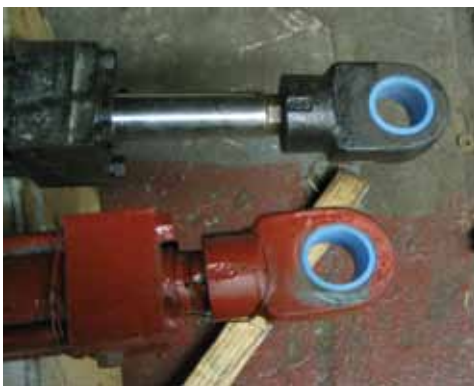
ThorPlas-Blue steering and linkage bearings installed
