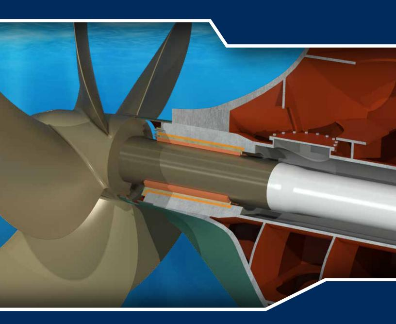
COMPAC OPEN SEAWATER LUBRICATED PROPELLER SHAFT BEARING SYSTEM FOR MERCHANT FLEET VESSELS
